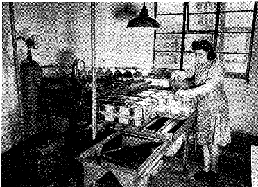
Fig. 13. Apparatus in which cans with dehydrated herring are gas-packed. The closed cans are pierced and introduced into a vacuum chamber where the air is removed. Nitrogen is then let in at a slightly positive pressure, and the cans are closed by soldering immediately after their removal from the chamber. (U.K. Ministry of Food, Crown Copyright).
