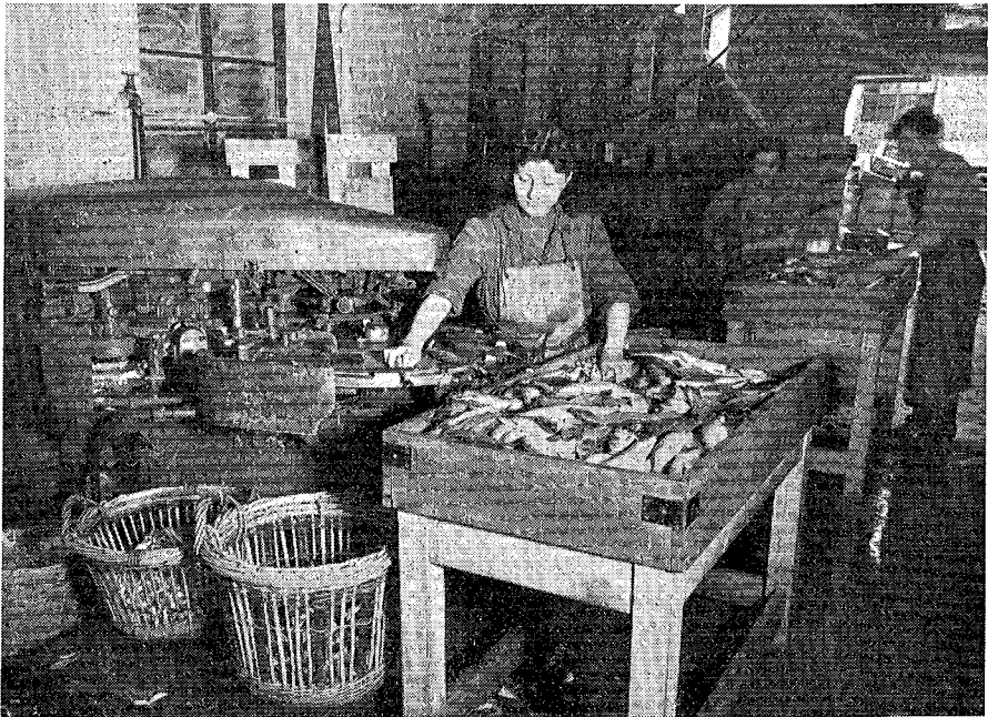
Fig. 5. Herring filleting machine in use in dehydration plant. (U.K. Ministry of Food, Crown Copyright).
