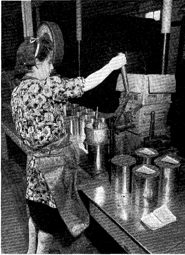
Fig. 12. The dehydrated herring material is packed under pressure into the cans. (U.K. Ministry of Food, Crown Copyright).
