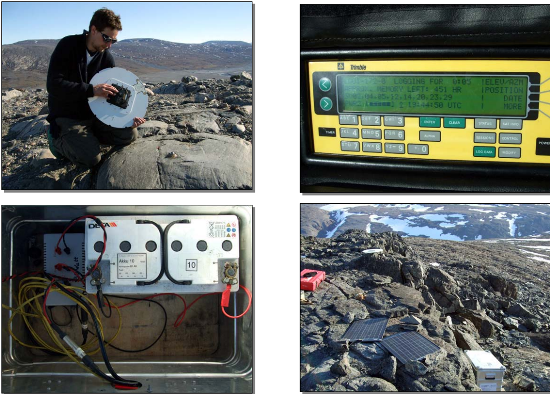
Fig. 7.1: Typical set-up of a GPS station.
