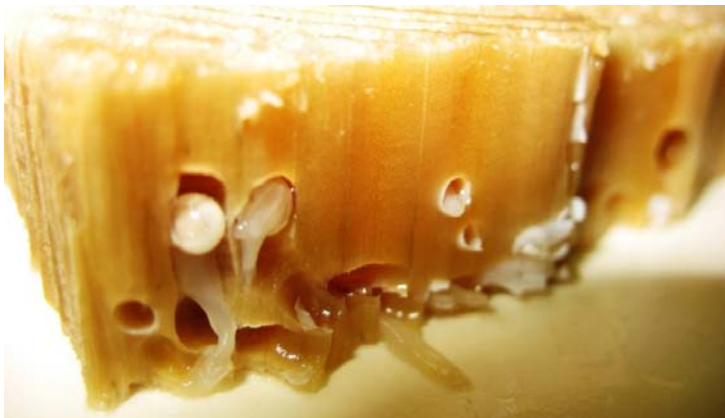
Figure 5.8.1: Partly degraded LOOME wood-cubicle with wood-boring bivalves.
