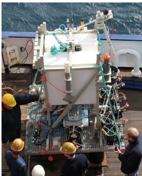
Figure 5.7.3.1: The figure shows the LOOME observatory frame right before deployment. The scanning sonar head can be seen on the upper right part of the picture characterized by the black rubber structure with the red cable attached.
