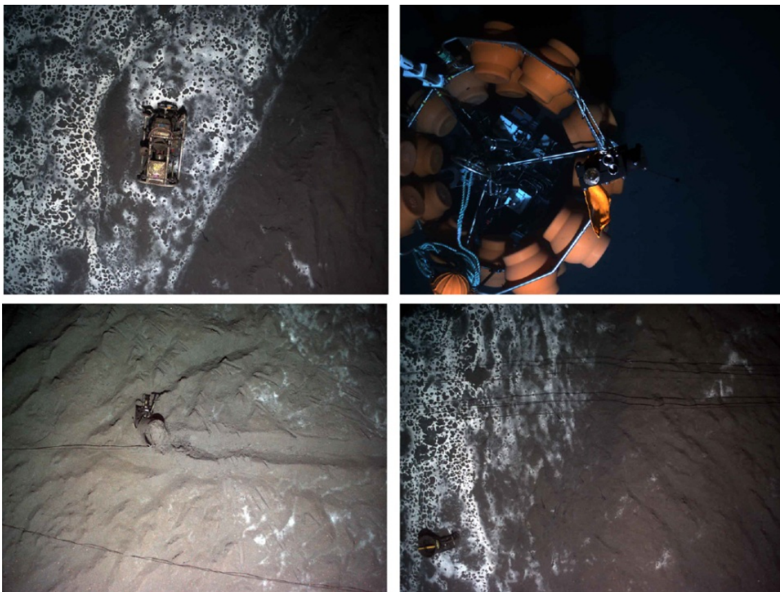
Figure 5.2.5.1: Examples of LOOME instruments deployed on the seafloor at the HMMV. Clockwise from top left: IFREMER time-lapse camera; MPI-Bremen Lander (3m tall, hence, photographed while Sentry flew just 2 m above the instrument at ~1260 m depth); LOOME T-sensor 1 (bottom left) with cabling for 4 additional sensors extending across image from left to right (~N-S); LOOME T-sensor 4 with cabling for LOOME T-sensor 5 continuing, left to right (N-S) across image. (Note the “scour” marks left behind by active mud flow toward the south in the “wake” of the T sensor).
