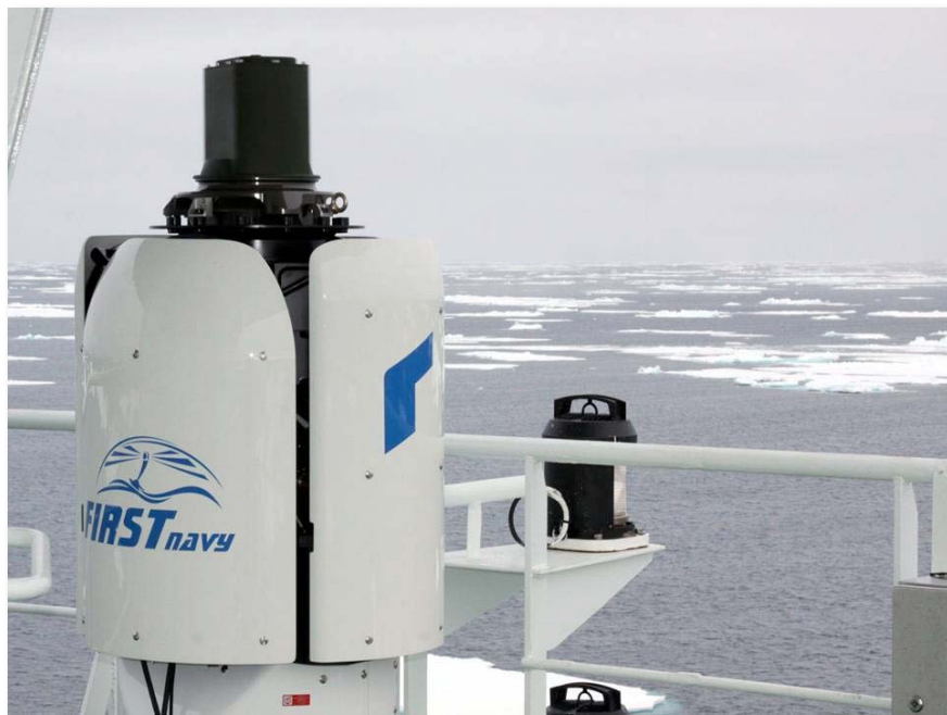
Fig. 5.2: FIRST Navy camera and gimbal on the crow's nest
