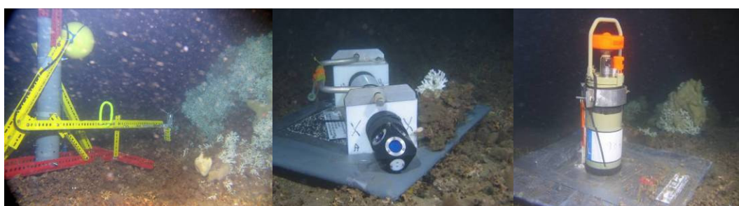
Fig. 4 Left: the velocimeter taking measurements at the coral reef. Middle: an upward looking ADCP. Right: Aanderaa RCM9 current meter with optical oxygen sensor positioned at reef floor.
