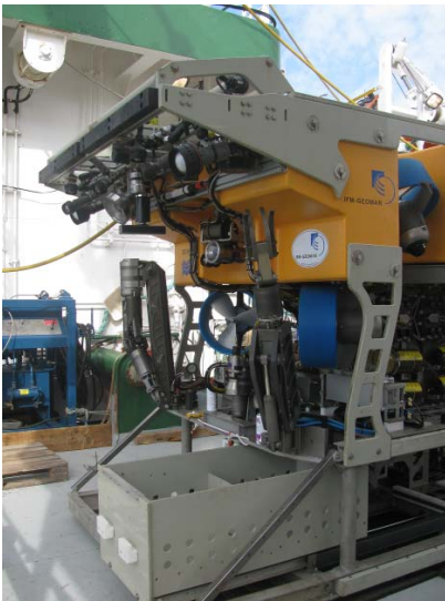
Fig. 5.1.1: Views of ROV Kiel 6000; left: front with cameras, manipulators and tool sled for storage of the push corers; right: starboard side with KIPS water sampler, CONTROS sensor package and FSI CTD.
