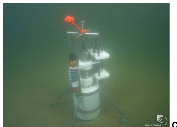
Fig. 5.1.5: Schematic drawings of the Pore Water Sampler (PWS). A: Overall setup with frame, B: Cross-section showing Rhizon lance and syringe carrier in penetration and operation modes, C: PWS with HOMER beacon deployed by ROV in the sandy sediments of the Southern German North Sea during CE0913.
