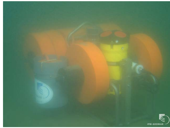
Right: The low profile lander deployed in the high bottom water current regime of the Southern German North Sea. Visible are the casings of the ADCP (yellow), the pressure sensor (white) and the recovery line (grey).
