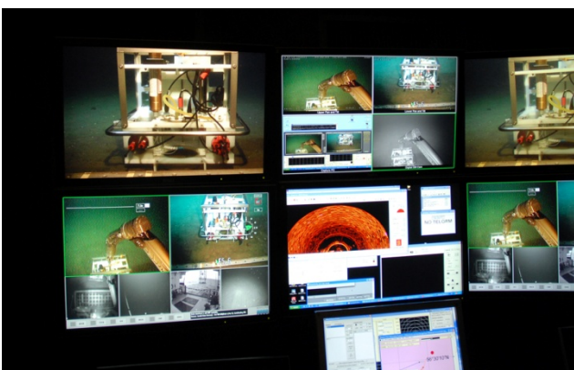
Fig. 5.1.6: View on the ROV console with the computer screens showing the different camera views, sonar and navigation data in the control van during deployment of the BC.
