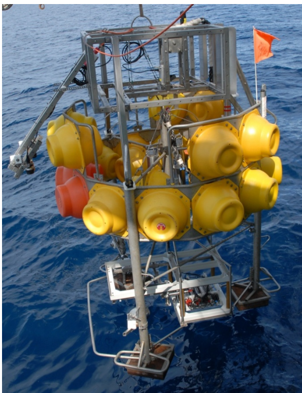
Fig. 5.2.1.1: Video-guided deployment of the Profiler Lander (PRF-L) is equipped with the microprofiler, a digital still camera system and 2 acoustic current profilers.
