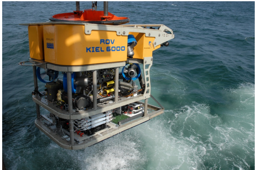
Fig. 5.1.1: Views of ROV Kiel 6000; left: front with cameras, manipulators and tool sled for storage of the push corers; right: starboard side with KIPS water sampler, CONTROS sensor package and FSI CTD.
