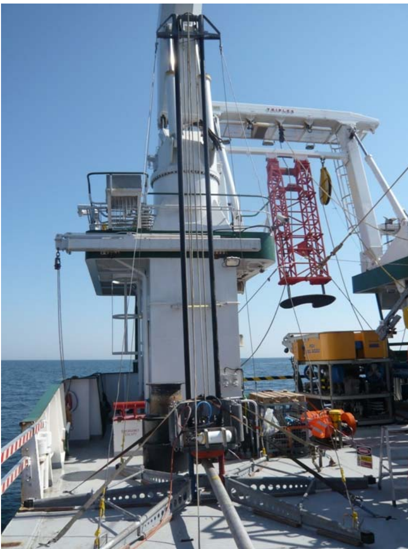
Fig. 7.1.1: Vibrocorer GEO 6000 operated from RV Celtic Explorer during CE0913.
