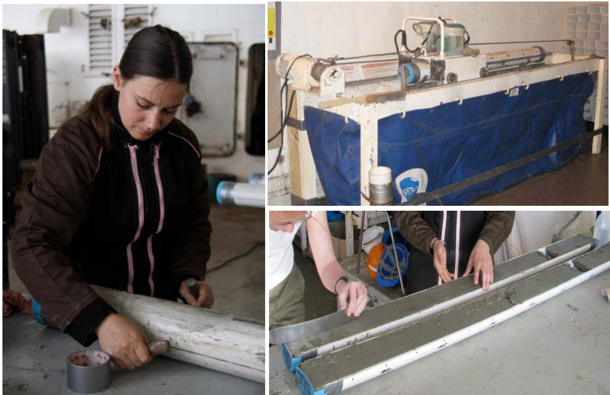
Figure 23: splitting system (top right). Charline separates the two halves with a fishing line (left) and half cores ready for sedimentary description (bottom right). Photos D. Catelain and M. Sadovnik.
