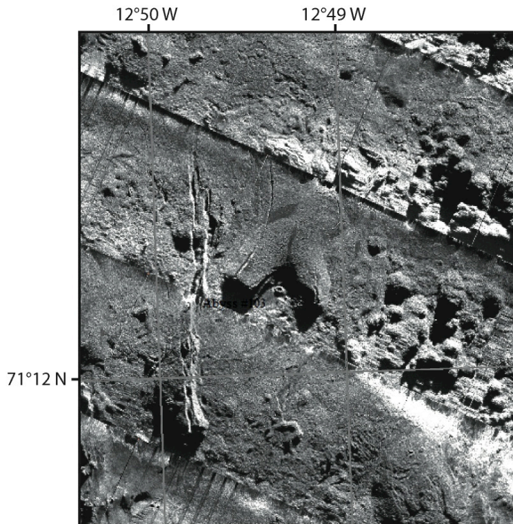
Figure 6.5: Sidescan sonar from Abyss #103 of a sheet flow on the axial valley floor. The large tumuli in the centre of the image may represent the location of the vent. Flow textures can be seen on the surface and hummocks on the right hand side.
