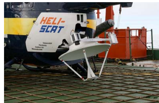
Fig. 3.2.2: Picture of the radar antenna looking out of the helicopter together with the IR camera (to the left above the antenna) and the Video camera (to the right above the antenna)
