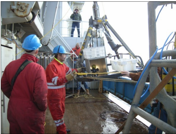
Fig. 5 Deployment of small ROV with "garage" mounted on former boxcore frame
