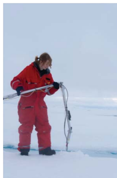
Fig. 3.13: Photograph of under-ice radiation measurements using a foldable holder, so called l-arm. Station on August 29 (78-227).
