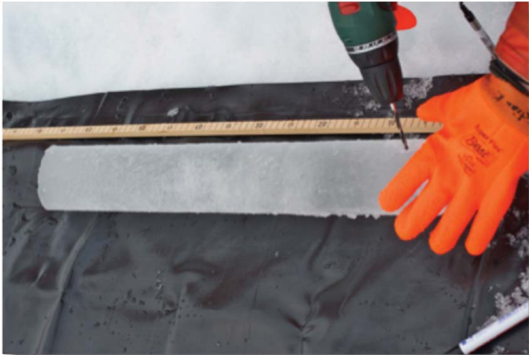
Fig. 3.18: Drilling of small holes in a sea ice core in preparation for temperature measurements every 10 cm
