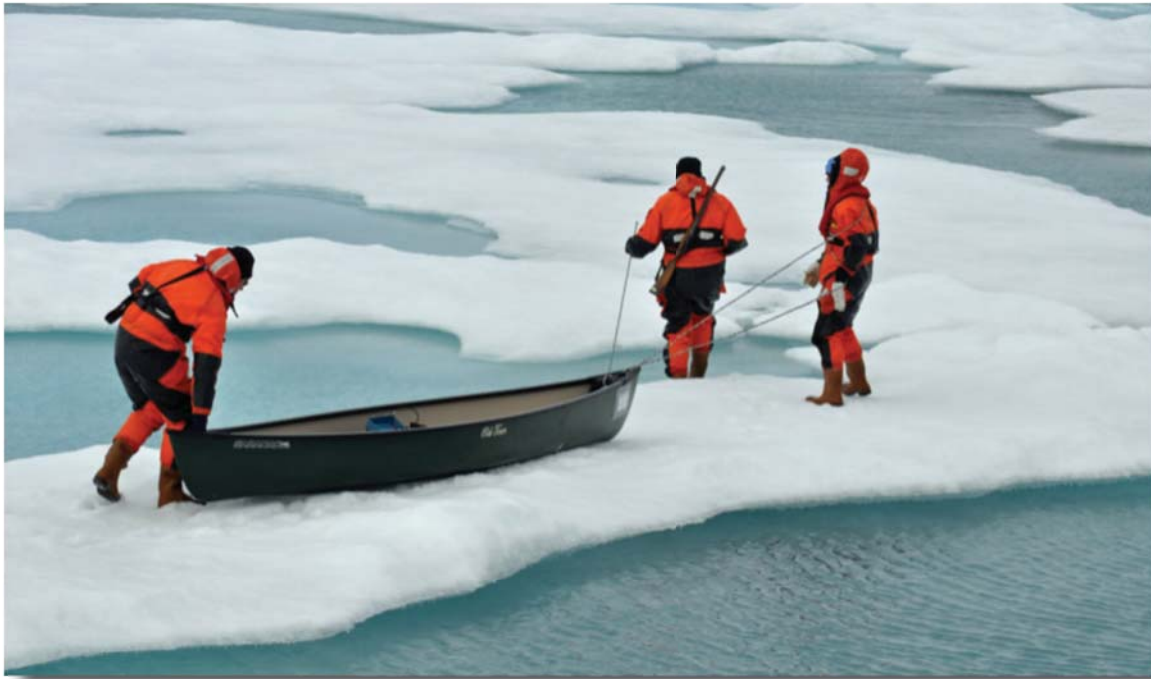
Fig. 3.23: Ground-based sea ice thickness survey with an EM31 Mk II (Geonics Limited). The instrument was towed over the sea ice in a canoe, which also allowed ice thickness measurements in melt ponds (Photo: Estelle Kilias).
