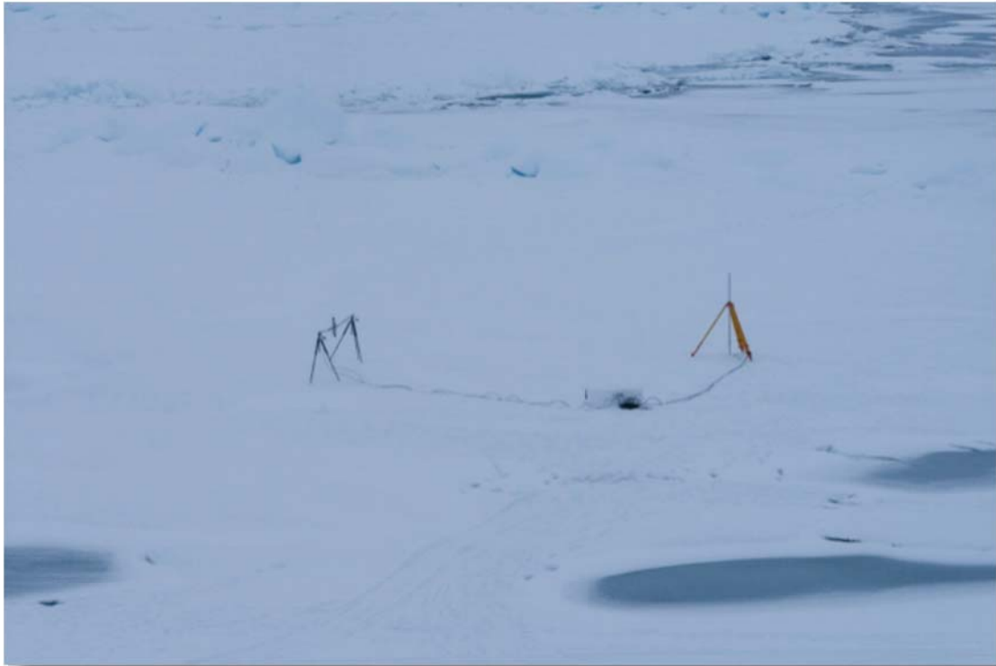
Fig. 3.12: Photograph of the radiation station. Two sensors are mounted above the surface for albedo measurements (left rack), one mounted on an l-arm held by the yellow stand, and two hanging under the ice at the position of the l-arm. Station on September 5 (78-238).
