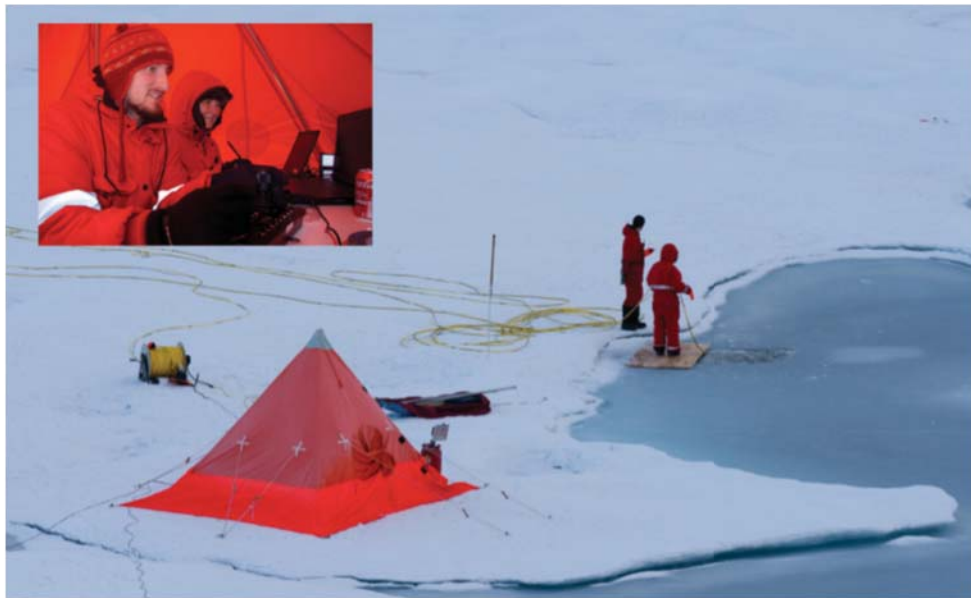
Fig. 3.11: Photograph of the ROV site taken from board Polarstern during the ice station on September 2 (78-235). The main picture shows the deployment hole in a frozen (surface) melt pond, the yellow tether, and the pilot tent. The inset picture shows two ROV pilots, one controlling the ROV and one controlling the sensors and documenting all operations.
