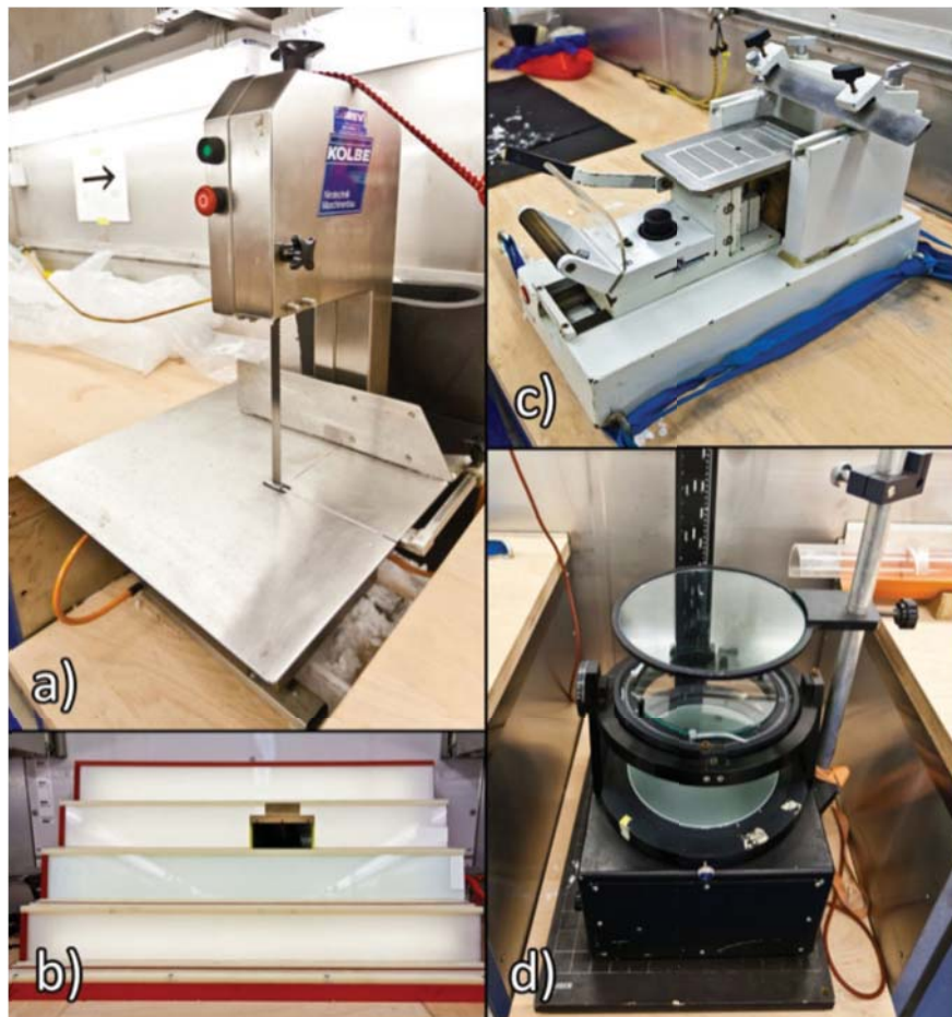
Fig. 3.21: Equipment for texture analysis of sea-ice cores. a) Kolbe K200 Band Saw; b) Light table with crossed polarizers; c) Microtome; d) Universal Stage.
