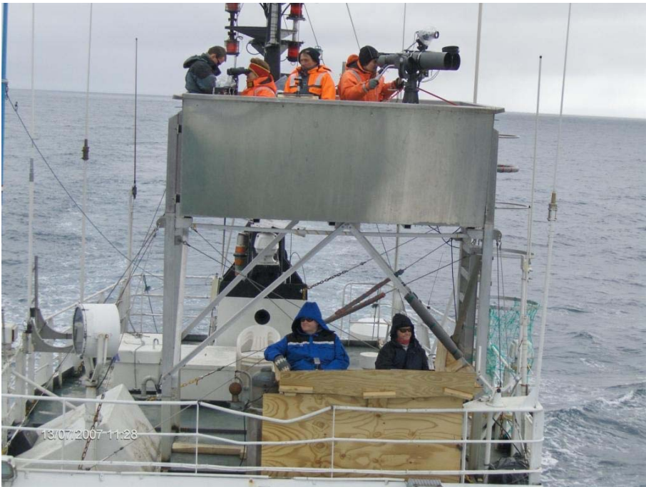
Figure 4. T-NASS Venus: View of the two platforms with the special anti-vibrating mounting of the tracker platform.
