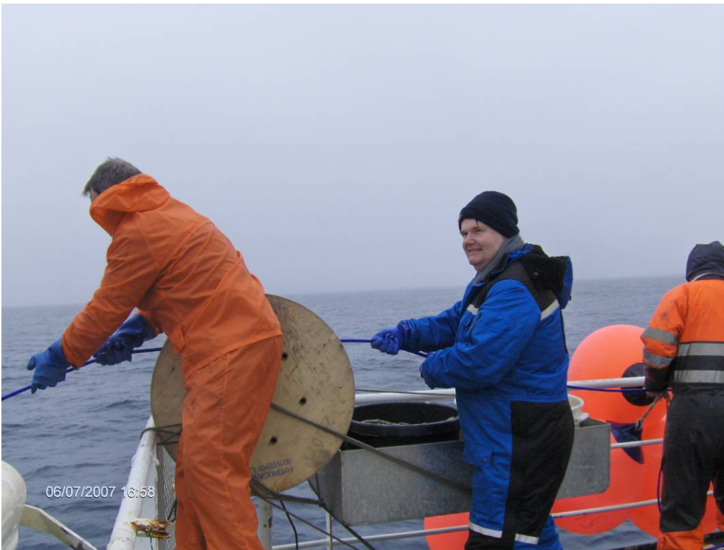
Figure 9. Pulling in the cable with the hydrophone (wooden drum used for protecting the cable).
