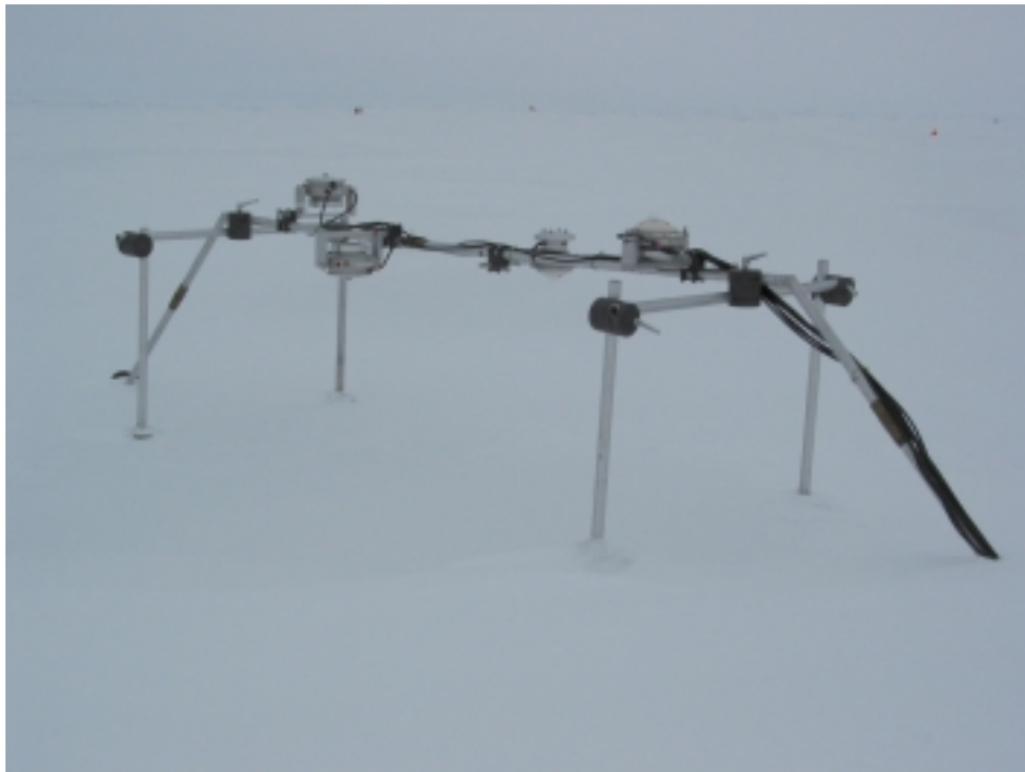
Figure 4.2..D Frame with the four radiation instruments. From left to right: upward looking long wave radiometer, downward looking long wave radiometer, short wave downward and short wave upward looking radiometer.
