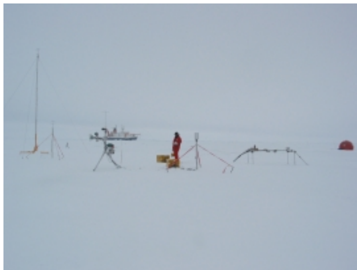
Figure 4.2.C: The surface layer measurement and instrumentation site on during the ice drift station. From left to right: 9m-mast and 2m-mast with Sonics, basic meteorological mast, in the background RV Polarstern, between them the 10m profile mast of FIMR, yellow boxes for electricity supply and data storage, precipitation gauge, frame with radiation instruments and tomato for storage of boxes, spades, fuel tanks and other equipment.
