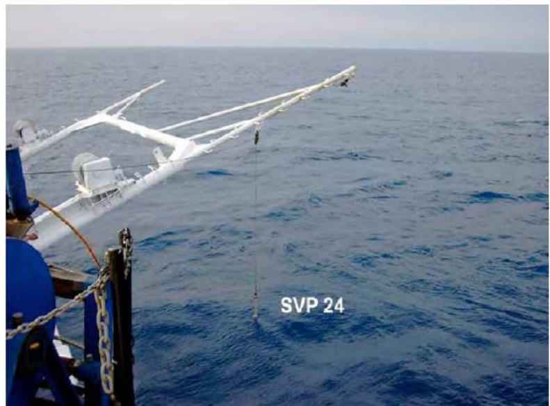
Fig.B. 4: The Sound Velocity Probe is usually deployed by lowering the portside frame.
