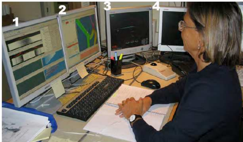
Fig. B.3: Navigation room. The surveyor also operates the MBES by means of PDS2000 suite. Monitors shown in the photo: real time navigation and acquisition control (1 & 2), MBES control (3 & 4)
