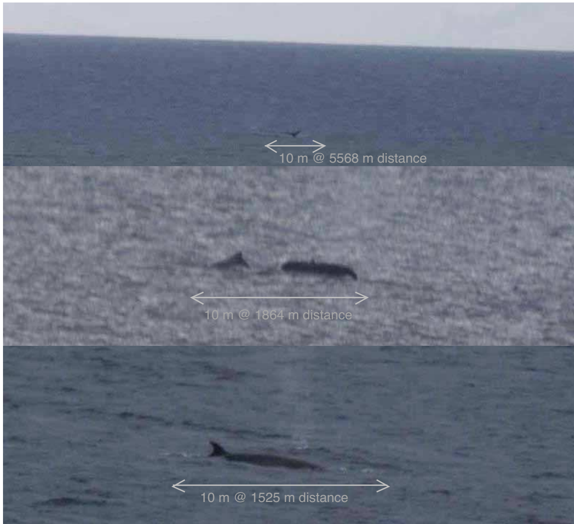
Fig. 5.2.2: Three examples of automatically triggered whale detections, which were captured by the PiP system. They could retrospectively be identified as humpback whales (top at 5,568 m distance and middle, 1,864 m) and a minke whale (bottom, 1,525 m).
