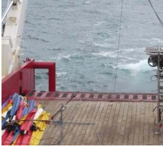
Figure 16. View of JCR's after deck during seismic operations, with the air from the most recent shot reaching the surface immediately behind the float.
