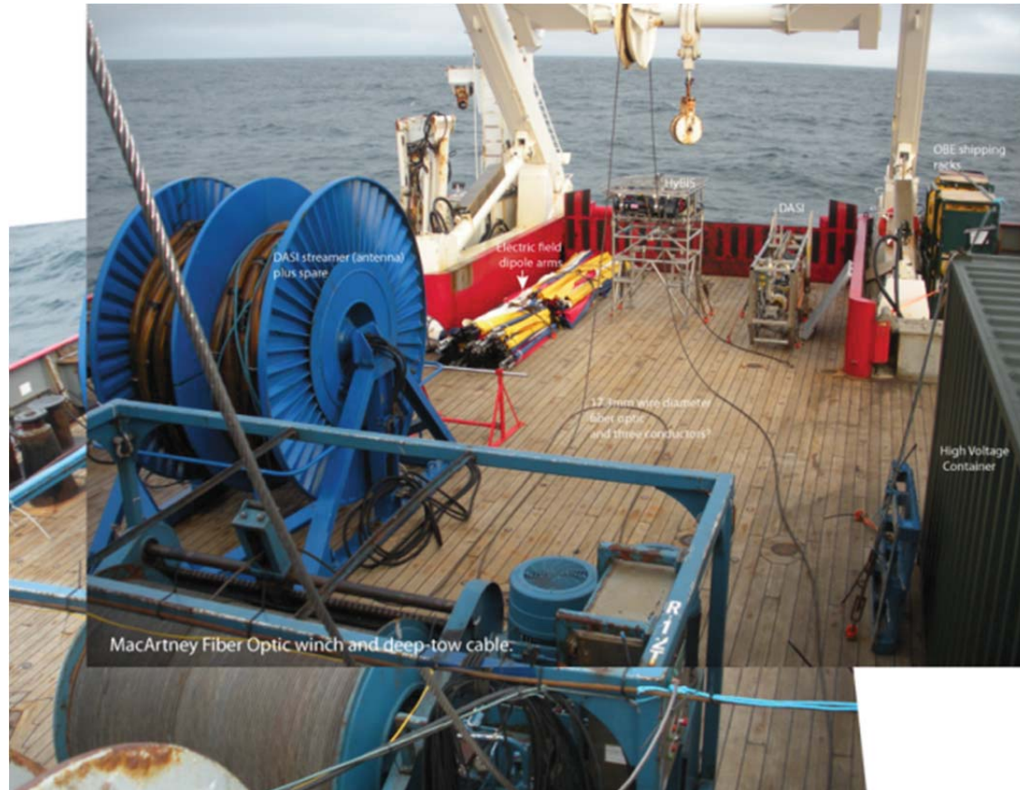
Figure 22. Layout of major items of equipment on the after deck of RRS James Clark Ross.
