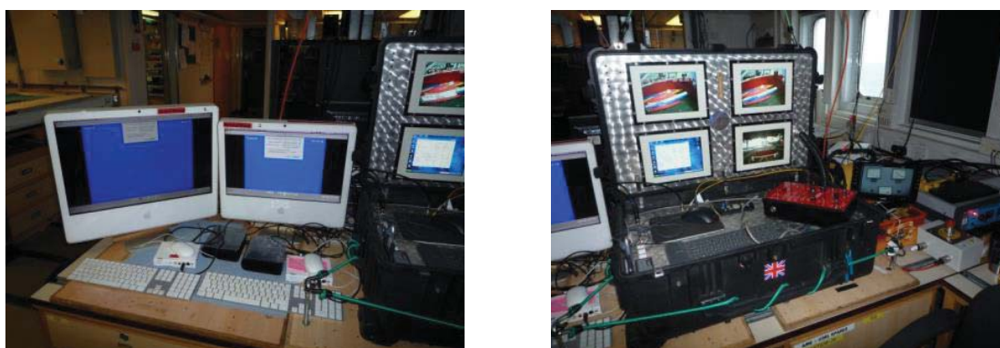
Figure 15. UIC Lab HYBIS control console setup, showing video screen arrangements (left) and the HyBIS video logging system and main control box (right)
