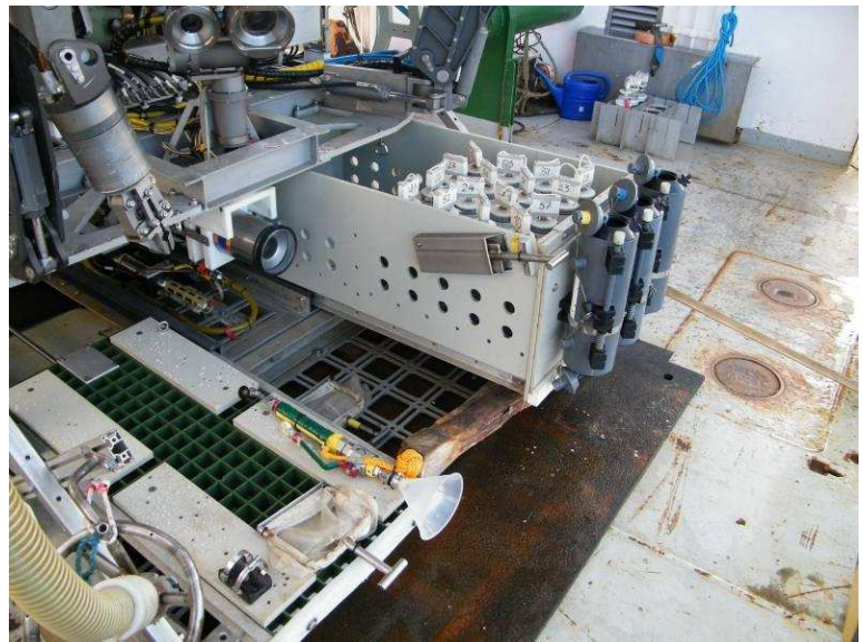
Fig. 4.4.2.2: ROV KIEL 6000 most common sampling set up with 16 push cores, 3 Niskin bottles, 2 nets and a gas-sampler on the front porch.
