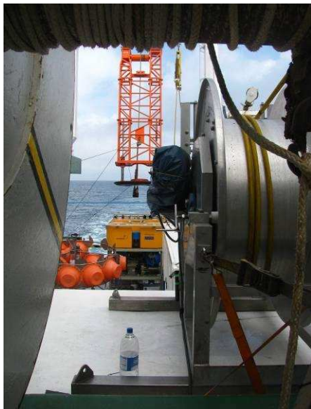
Fig. 4.4.2.1: Decks-setup of ROV KIEL 6000 system using a 500 m tether cable (see right on capstan winch).
