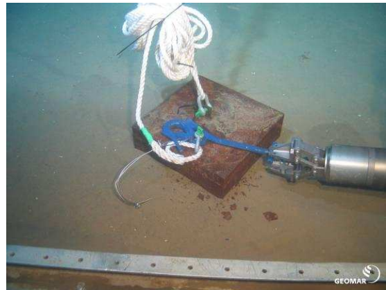
Fig. 4.4.3.1h: Hook-wire-construction for recovering ADCP and anchor weights.
