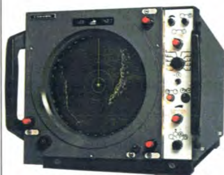
MARINE RADAR FR-1011 3 cm (X-Band) 72 n.m. rekkevidde
