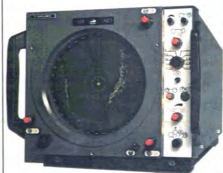
MARINE RADAR FR-1011 3 cm (X-Band) 72 n.m. rekkevidde
