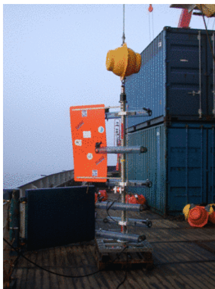
Bottom Water Sampler applied for investigation of concentration profiles close to the sediment water interface.
