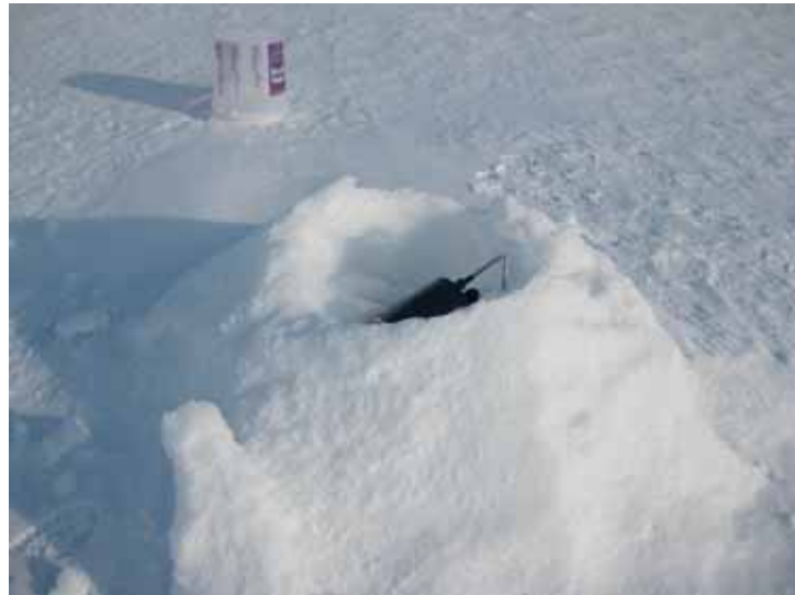
Fig. 3.2.5: Station Lena1-2 after the visit of a polar bear. The frozen snow heap was opened and the plastic bucket lifted and set down beside the heap. The seismometer was tilted when the bucket was lifted. Picture was taken during the recovery of the station on 31/08/09.
