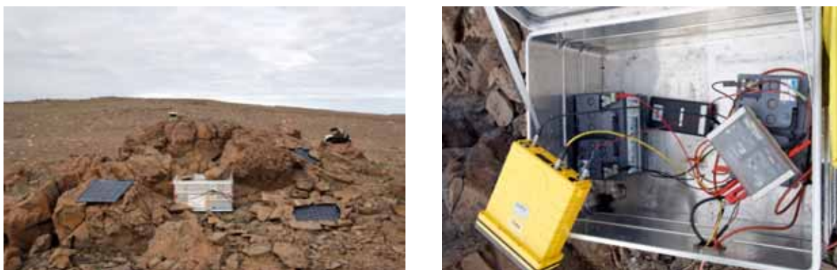
Fig. 4.1: Typical set-up of a GPS station.
