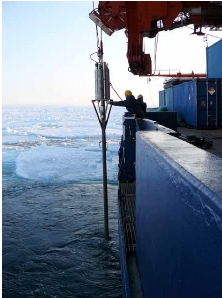
Fig. 3.3.3: Heat flow measurement in the ice.
