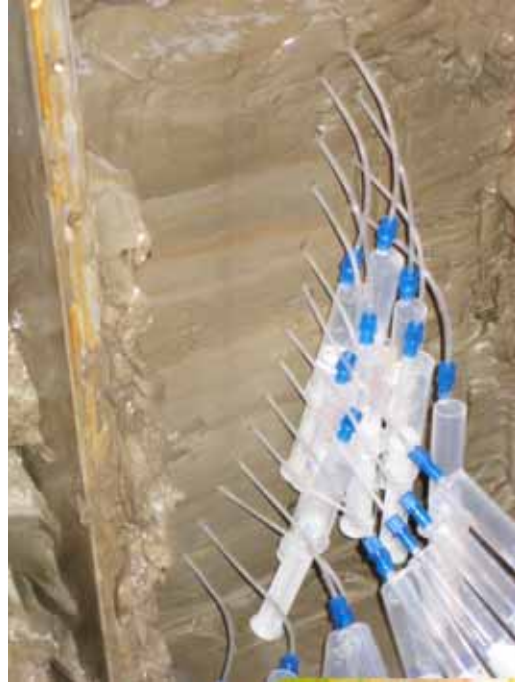
Fig. 40: Giant Box Corer on the working deck, sampled with rhizons and plastic syringes. Colour changes probably related to different sedimentary Mn contents are clearly visible.
