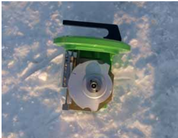
Fig. 66: 24 Hours Assembly with coated Sampling Slide
