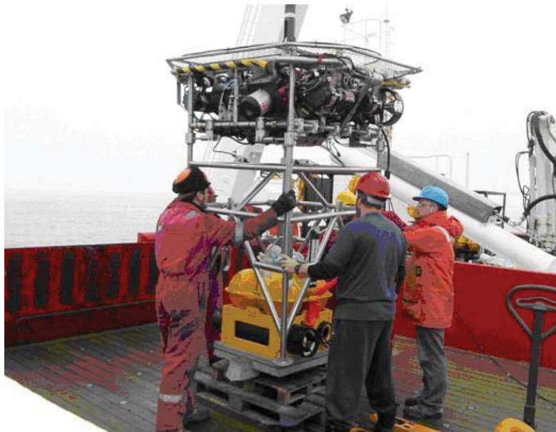
Figure 11.7: Securing the OBS to HyBIS
