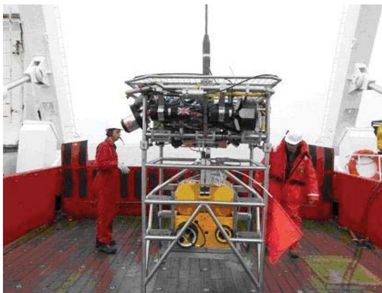
Figure 11.6: OBS Secured to HyBIS with bent flag and radio beacon antenna
