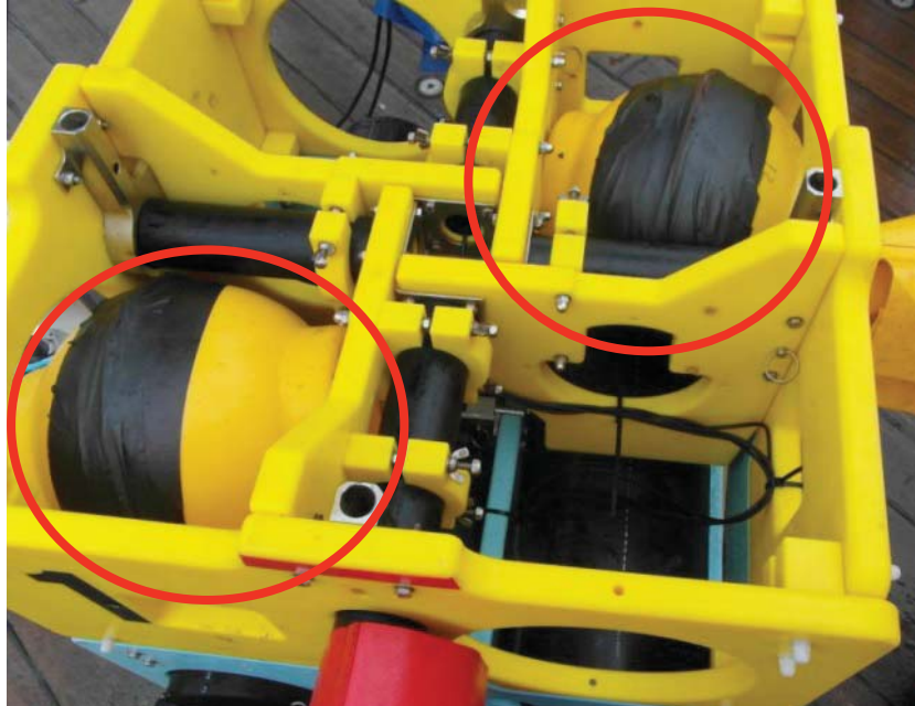
Figure 11.3: Floats mounted inside the EM Chassis
