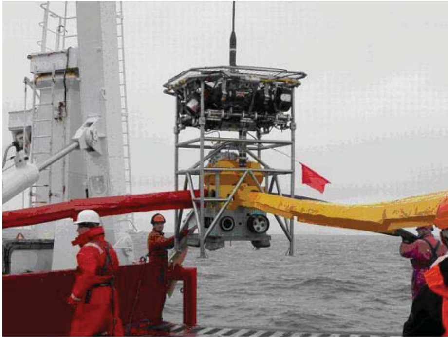
Figure 11.18: Deploying EM Instrument with HyBIS
