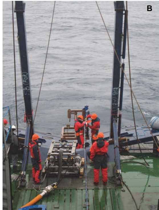
Fig. 19 A. Large airgun array of two linear arrays consisting of two 520 cu. inch G-guns each. The total volume of this array is 2080 cu. inch. B. Launch of the streamer. Birds are installed on the streamer for depth control. A US fender used with the airgun array can be seen to the right (grey).
