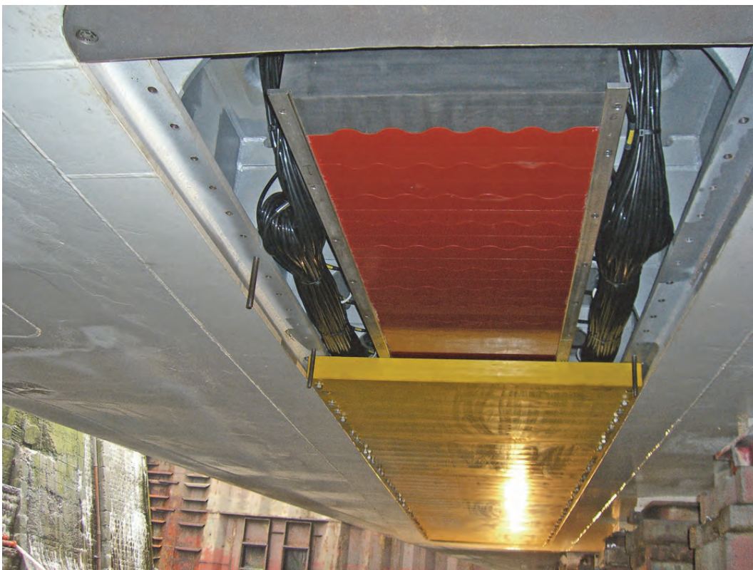
Figure 7. EM122 Tx transducer during installation, with some of the ice protection elements fitted.
