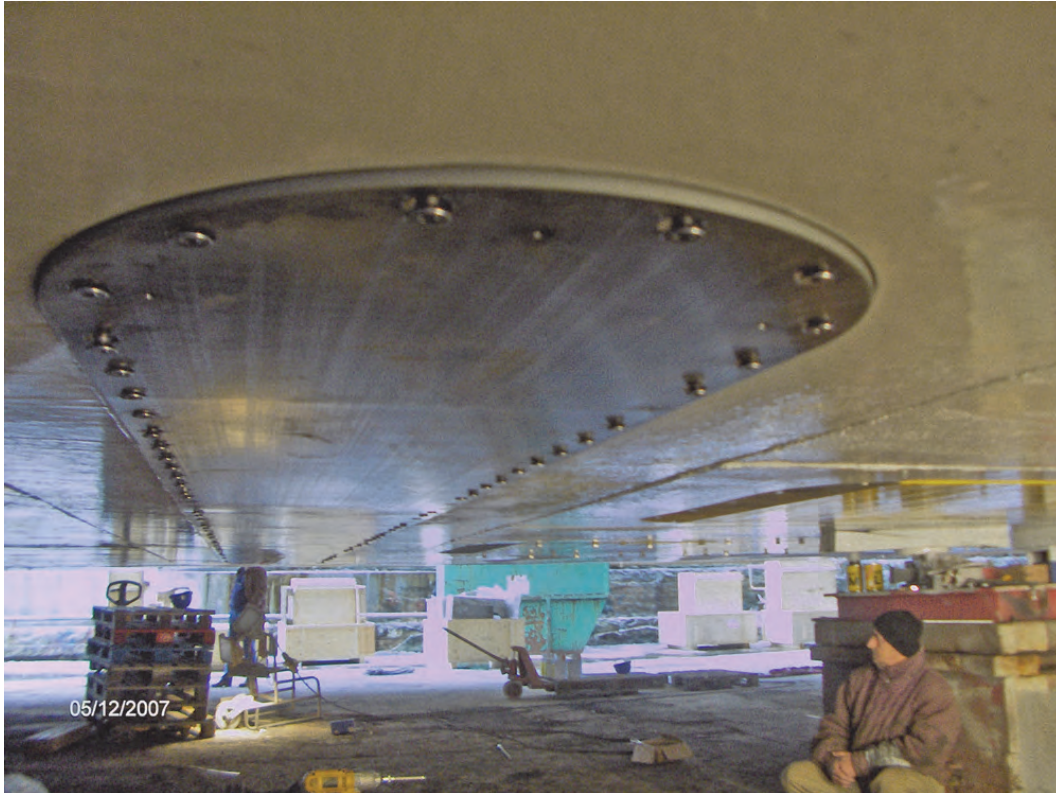
Figure 6. EM122/SBP120 Rx transducer during with titanium plate covering ice protection elements.
