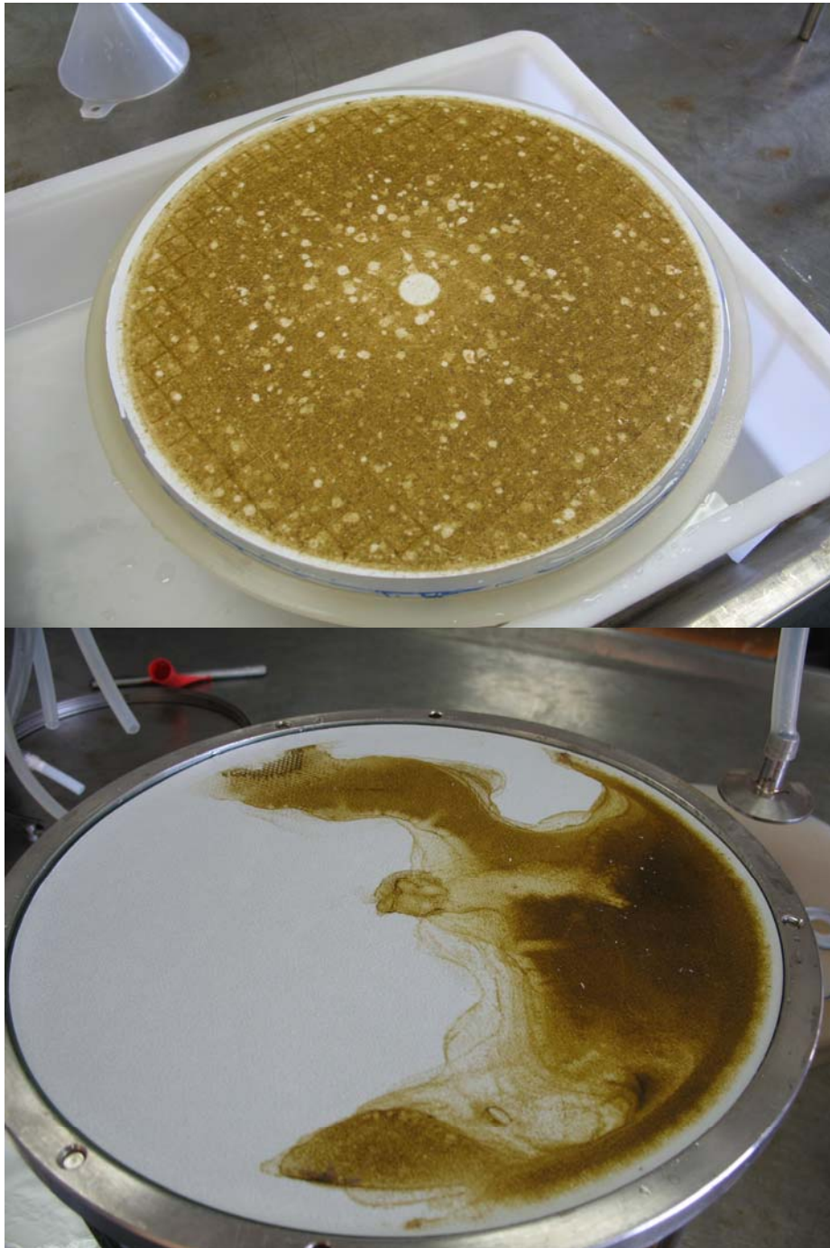
Fig. 11. The GFF filters containing samples and ready for extraction. The upper filter is from the automated in situ pump; the lower filter is from the tabletop filtration unit. Note that the samples were taken at different stations.
