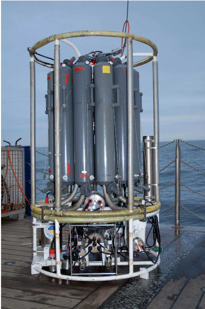
Fig. 11: Water sampler (12x10 L Niskin ) rosette including SBE9plus CTD, pH sensor (SBE27), and the HydroC/CH 4 /CO 2 /PAH sensor package with power pack. The orange cable attached to the winch cable is connected to the digital video telemetry system.
