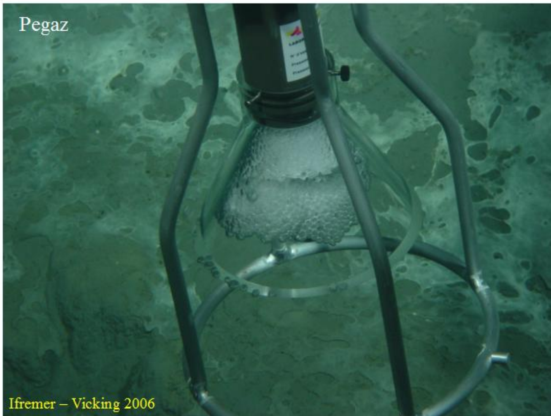
Figure 6.6. : Pegaz sampling system, filled of methane bubbles coated with gas hydrates on the HMMV
