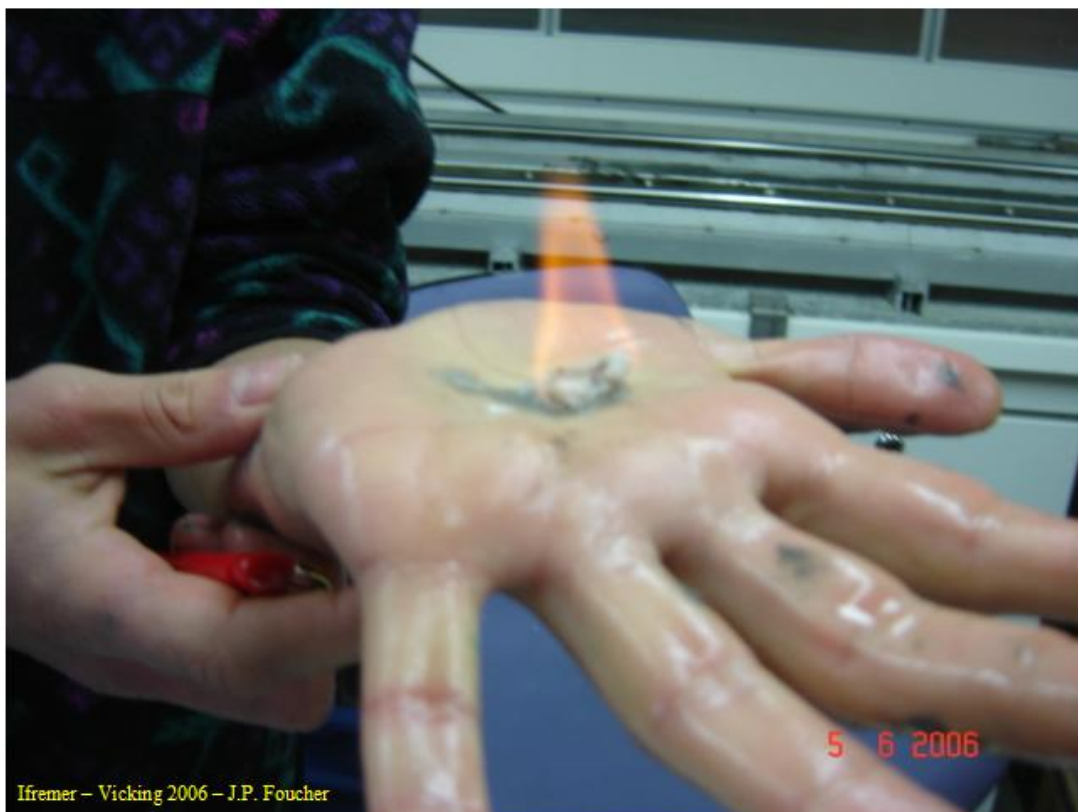
Figure 6.6. : Pegaz sampling system, filled of methane bubbles coated with gas hydrates on the HMMV
