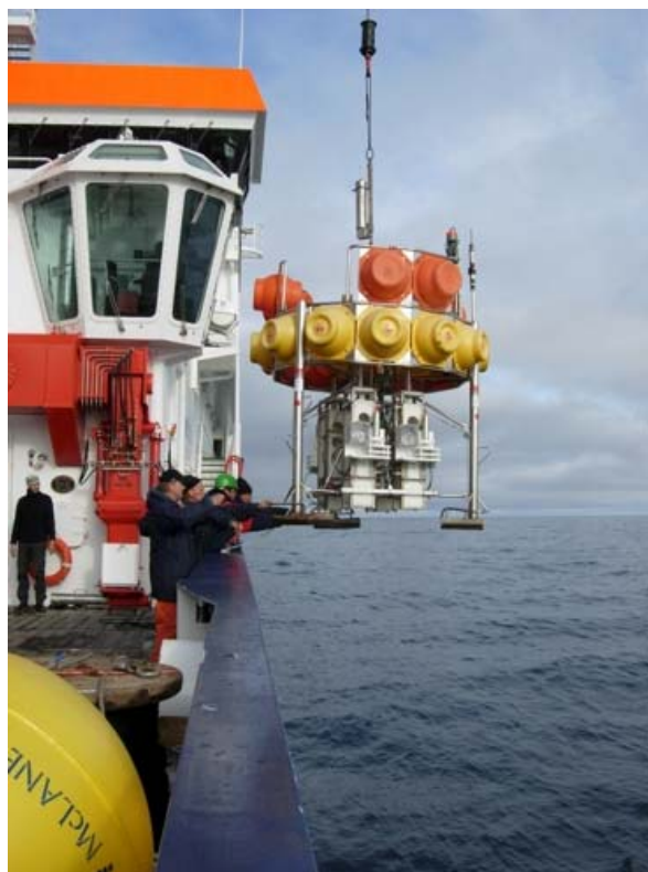
Fig. 4.16: Deployment of the free-falling grab respirometer
