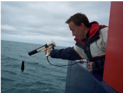
Fig. 1.9: An XBT is launched
