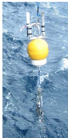
Fig. 1.4: The free-fall CTD (SBE 19) conceived by P. Le Grand, O. Peden, O. Ménage and S. Leizour
