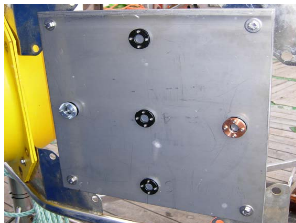
Fig. 4.18: Plastic panel with silicon coating (a) and five pieces of glass partly with coatings and different metal ring mounted on a metal panel (b)
