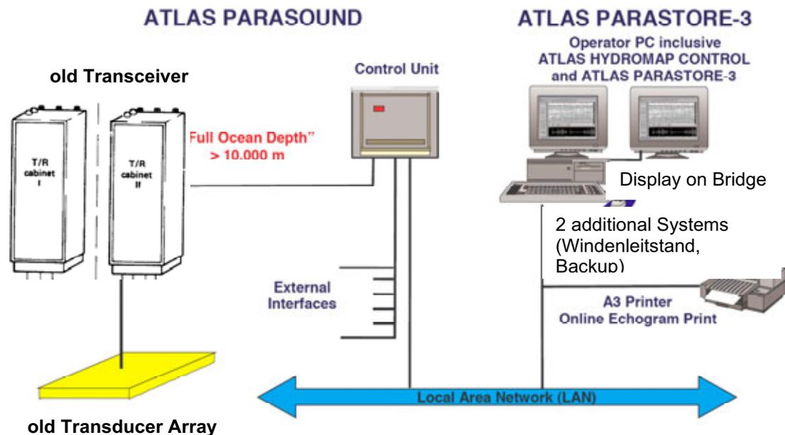
Figure 2: System architecture of new ATLAS PARASOUND DS2 system (2004) with communication over local area network.
