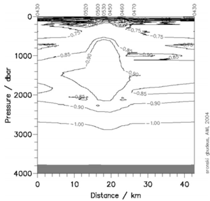
Fig. 4.3 Temperature along a transect across the coherent eddy
