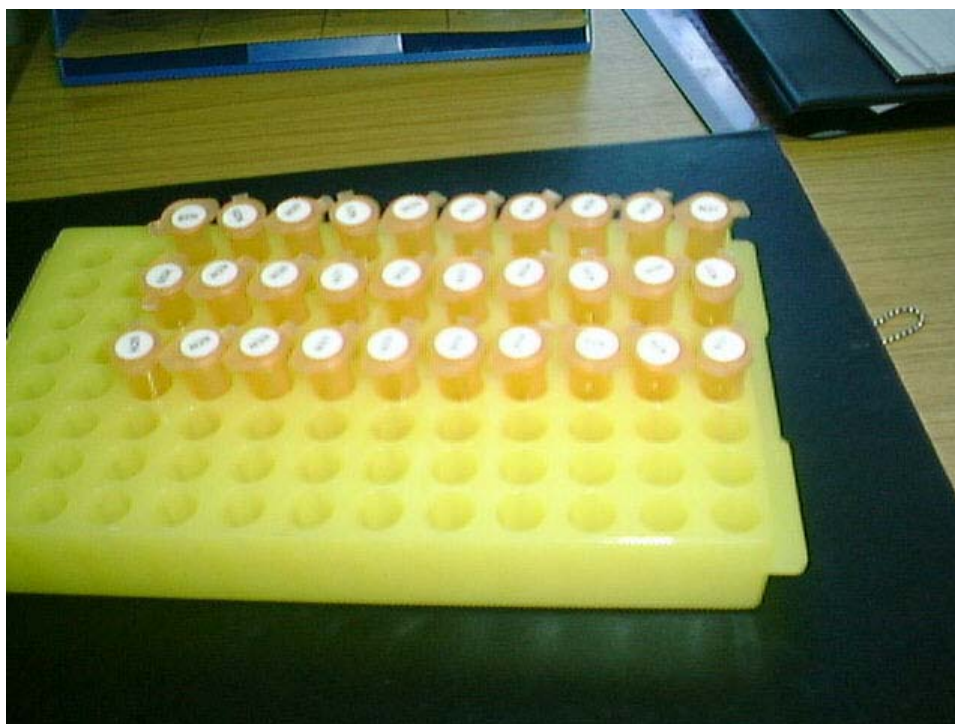
Figure 3.4.6.2 Picture of a rack holding Eppendorf like tubes for 10 fish with 3 replicates identified by spot labels on the lids. During storage a lid fits on top of the rack to keep the tubes in order during transport.
