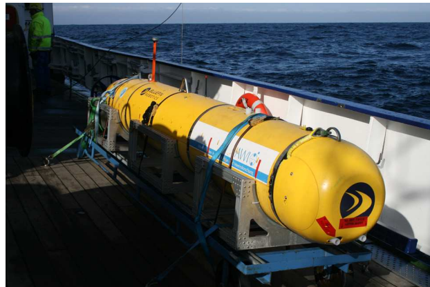
Fig. 5.3.1: AUV (AWI) for water column studies above the seafloor
