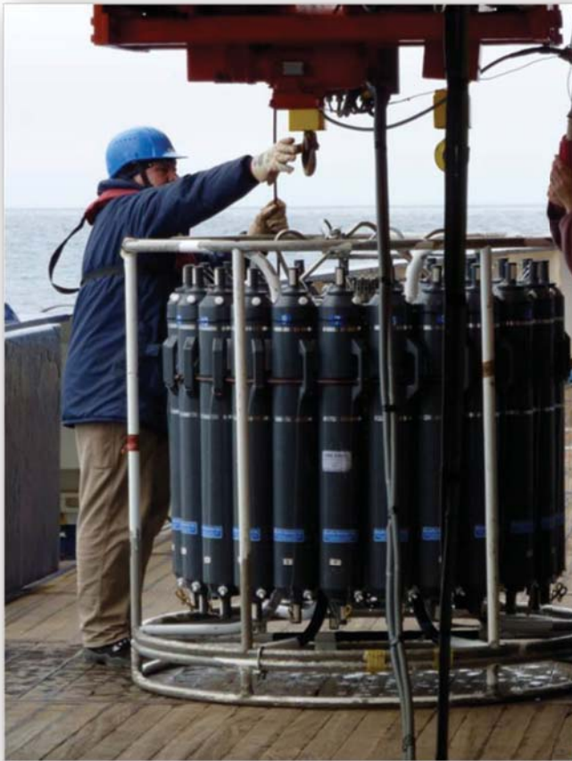
Fig. 3.1.1: Recovery of the CTD/Rosette at HAUSGARTEN observatory
