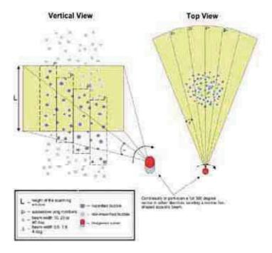
Fig. 3.6.1: The sketch shows the operation procedure for forward-looking sonar. The Imagenex 881a sonar-head has a rotating system providing the capability to obtain a full 360 degree sector scanning. The sonar measures the scatter intensities from objects by sending a narrow fan-shaped acoustic beam.
