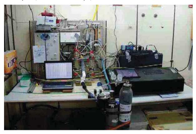
Fig. 3.2.1: Image of the set-up for continuous methane and carbon dioxide measurements on board R/V HEINCKE Cruise HE-387.
