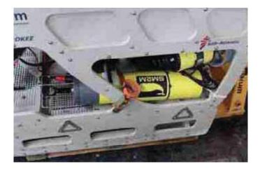
Fig. 4.8.6: Hydrophone set up on the ROV.
