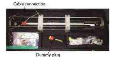
**Fig. 3.1.6:** Image of the sound velocity probe on R/V HEINCKE.
