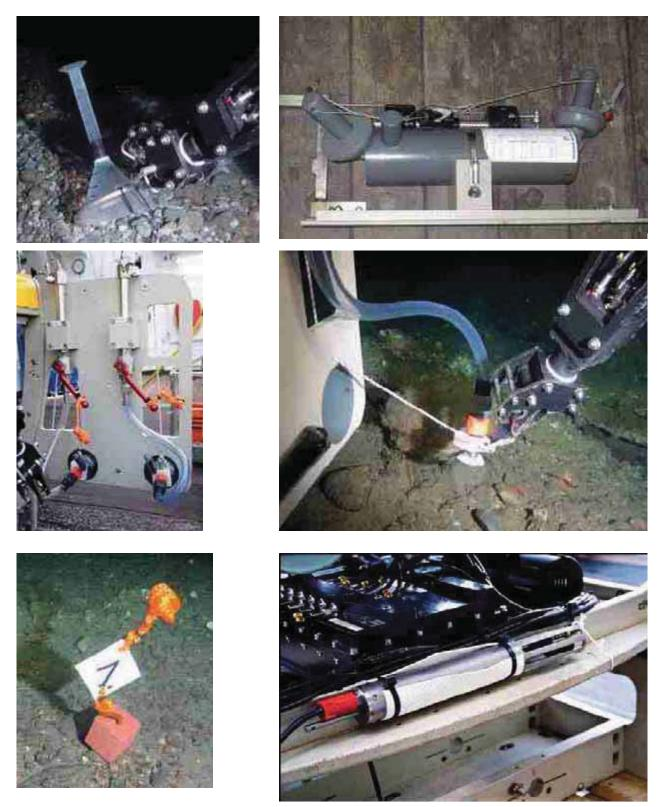
**Fig. 3.4.3:** ROV Cherokee scientific payload: (upper left) bubble catcher (2<sup>nd</sup> version), (upper right) Niskin bottle manufactured by Hydro-Bios, (middle) gas bubble catcher, (lower left) marker, (lower right) CTD mounted at the back of the vehicle.
