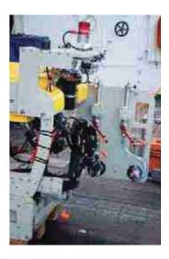
Fig. 3.6 2: The picture shows the front of ROV Cherokee with the Imagenex sonar on the top.
