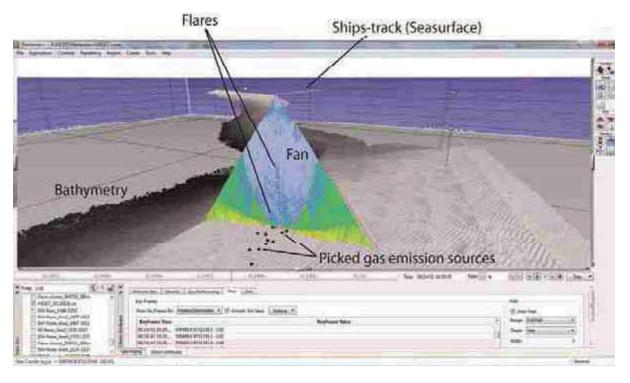
Fig. 3.1.2: Replaying fan in the 3D view of Fledermaus together with the achieved bathymetry.
