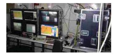
Fig. 3.4.2: The TCU in the drylab: to the left, the two cases with the monitors and to the right the 19" rack. The remote controls for the vehicle and manipulator are seen in front of the monitors.
