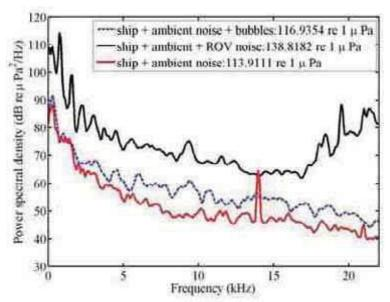
**Fig. 4.12.1:** Power spectral densities from hydrophone recording of Dive 03 during different sequences.
