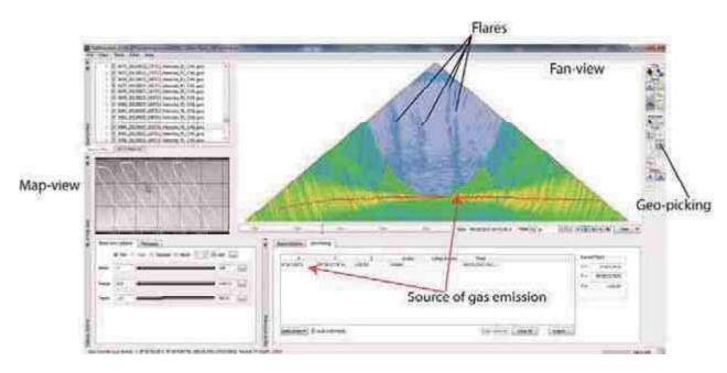
**Fig. 3.1.1:** FM Midwater tool to display the fan in 2D and convert the sonar files into \*sd files which can be opened with IVS 3D Fledermaus.
