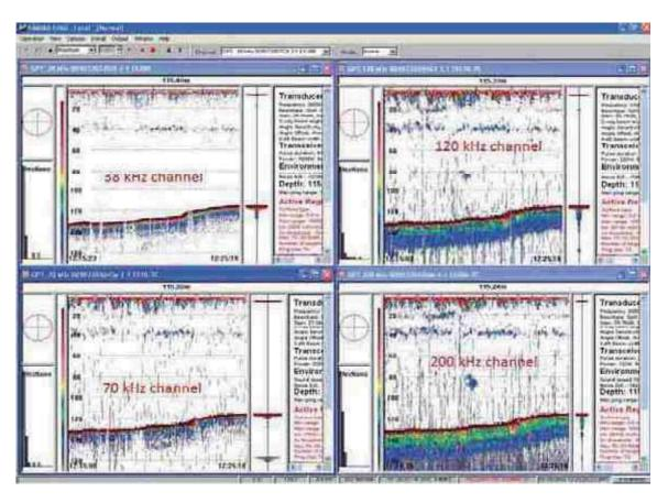
Fig 3.1.3: Overview of the ER60 interface showing the four channels that were available (Sv levels).
