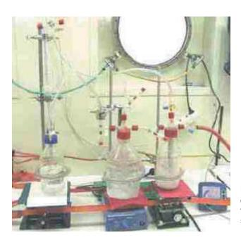
**Fig. 3.8.1:** Installation of the gas high-grade vacuum extraction system on board the R/V Heincke.
