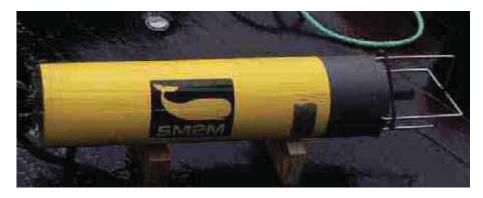
Fig. 3.7.1: Picture of the SM2M unit that was used for collecting passive acoustic data of bubble streams.
