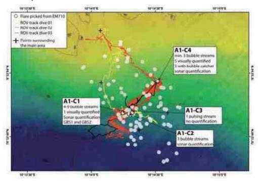
Fig. 4.8.3: Map of the dive area. Cluster A1-C2 with was documented first (sonar and visual quantification). The second part of dive took place in A1-C4 cluster where several gas bubble plumes were quantified.
